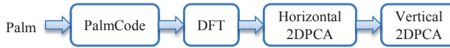
Fig. 5.2: Flow chart of the proposed method. (DFT - discrete Fourier transform; 2DPCA - two-dimensional principle components analysis)
